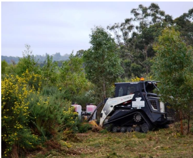
The Eco Blade in operation in 2 meter high gorse.
